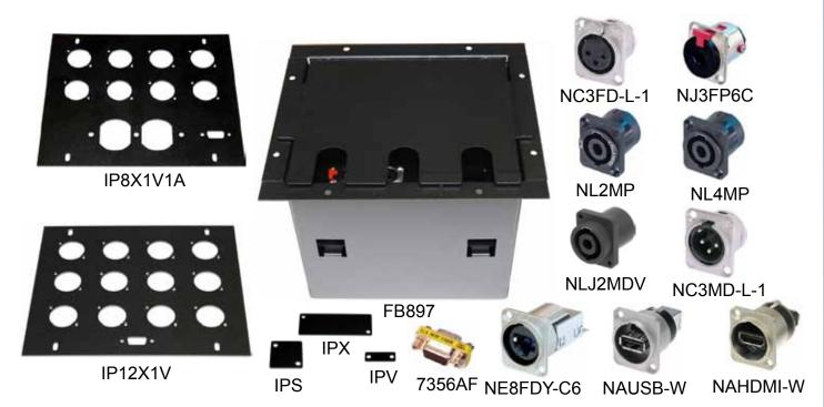
The FB897 Floor Box is a steel unit for installation in stage or church platform floors. It can be configured to provide many different combinations of microphone, monitor speaker and computer VGA connections as well as AC power.
