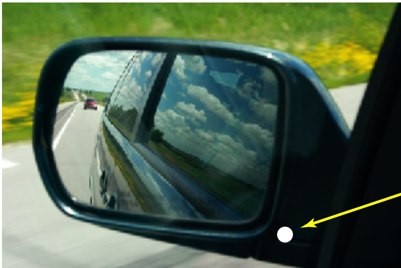
Microphone facing away from water source
